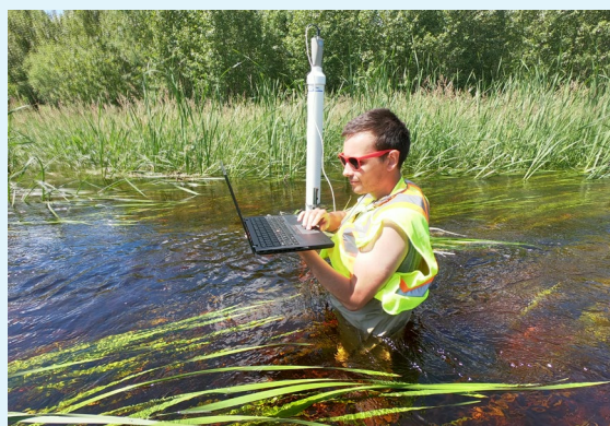
Figure 2. Manual flow (left) and automated water elevation (right) measurement at the De Salaberry water retention site
